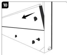
To remove the boards – ¼ turn all system locks to loosen, then one board at a time turn the locks fully anticlockwise. Standing in the middle, lean forward until the board pops off. Repeat as necessary. For the bottom board shake and lift out.
