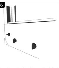
Place the bottom board into position behind the frame corner guide plates.
