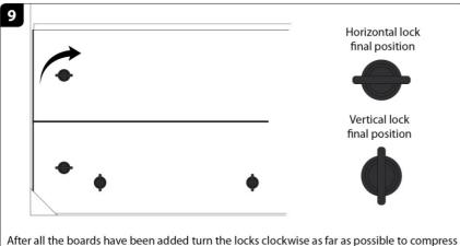
After all the boards have been added turn the locks clockwise as far as possible to compress the gasket and create a watertight seal. If system includes a top rail(s), remove frame caps and position rail end spigots into the frame.
