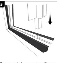
If the system includes a centre mullion post or intermediate posts, position post spigot into socket.
