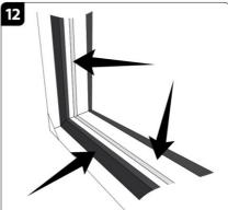
Routinely remove the treadplate(s) and poly-foam insert(s). Wash clean or vacuum the frame and gasket seals to remove dirt build up.
