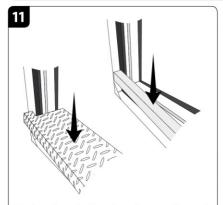
Replace the poly-foam insert, ensure the end slits locate over the corner plates so there is no gap between the insert and the bottom gasket. Replace the cover treadplate(s).
