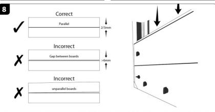
Add further boards, ¼ turn the locks each end to loosely locate pawls so the board cannot fall off. Click and fix together by pressing down hard one end, continue to press along the length in small steps until the boards click fully together. Check boards parallel and no gap.
